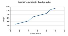
Fig. 9: Superframe duration with 4 anchors for localization
