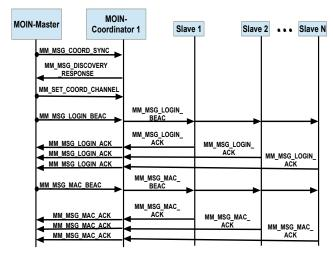
Fig. 6: Communication sequence realized by the MOIN Component Interaction Protocol
