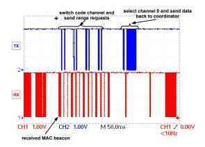
Fig. 8: Timing of a slave node with four ranging measurements
