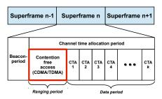
Fig. 4: Modified MAC superframe structure
