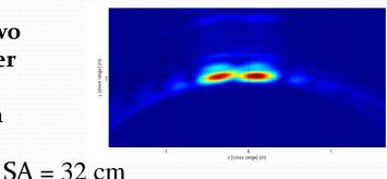
Increasing aperture (SA), the distance travelled by the radar, allows differentiation of two closely located targets.
