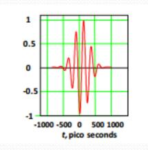
Greater distance between two pulses results in phase differences that create destructive and constructive interference
