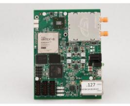
Figure 4. Photograph of the P400 UWB platform (75mm x 100mm).
